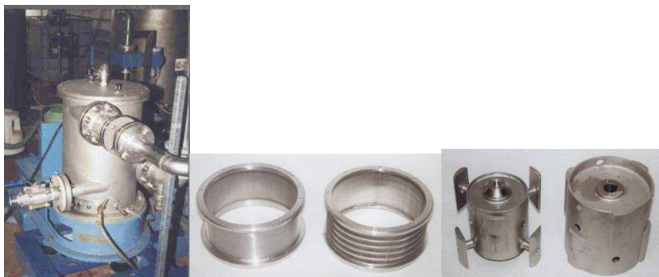
Figure 3: Pressure screen, screen baskets and rotor with foils for the pressure screen in the PTS pilot plant.
