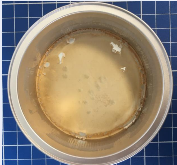
Gravimetric evaporation residue (filtrate acc. to Capi recyclability lab test method, V2)
