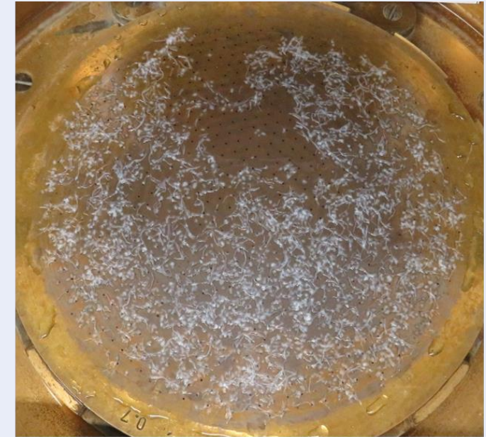
Reject of different barrier papers after 20 min disintegration (PTS-RH 021 method, 0.7 mm hole)
