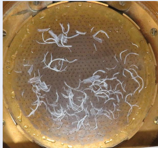
Reject of different barrier papers after 20 min disintegration (PTS-RH 021 method, 0.7 mm hole)
