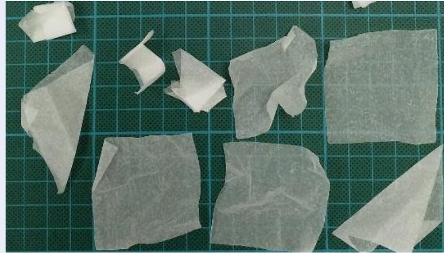
Reject of one-side PE-coated board after 20 min pulping
