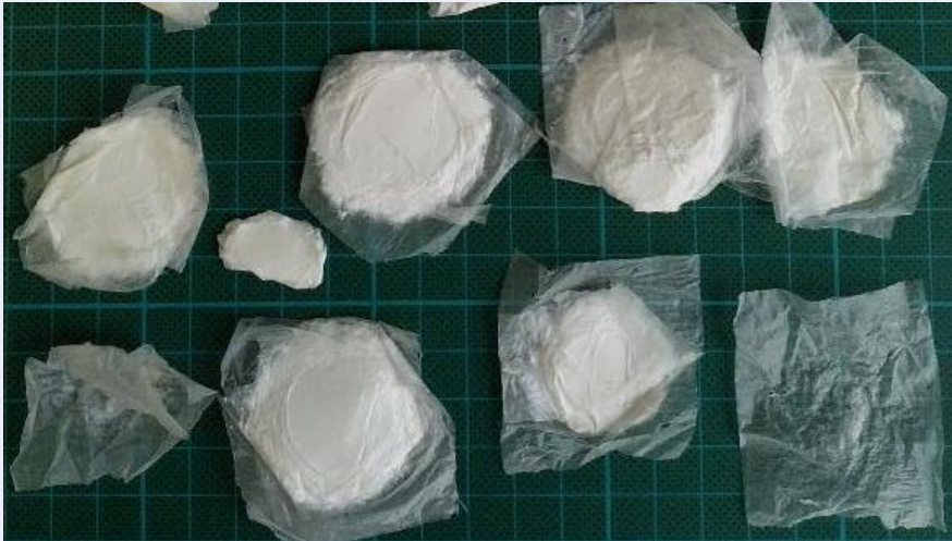
Reject of double-sided PE-coated board after 20 min pulping
