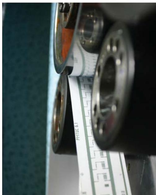
Fig. 1: Printing of SD structures; web width 35 mm
