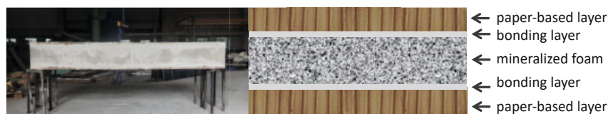
Fig. 2: Real and schematic sandwich element demonstrator structure
