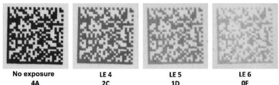
Fig. 3: Impairment of code gradings by different light exposure times (LE4 - LE6)
