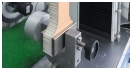
Fig. 1: Tensile test unit for paper structures of different thicknesses and compositions
