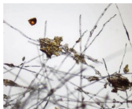
Fig. 2: Post-solvolysis aramid fibres showing small amounts of remaining resin deposits. In case of successful process optimization, new value chains can be created between aircraft industry and special paper manufacturers.
