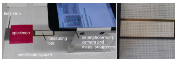
Fig. 1: Measuring set-up, enlarged view of measuring tool with coordinate system.
