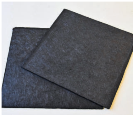
Fig. 2: Organo sheets made of hybrid nonwovens (source: Cetex)
