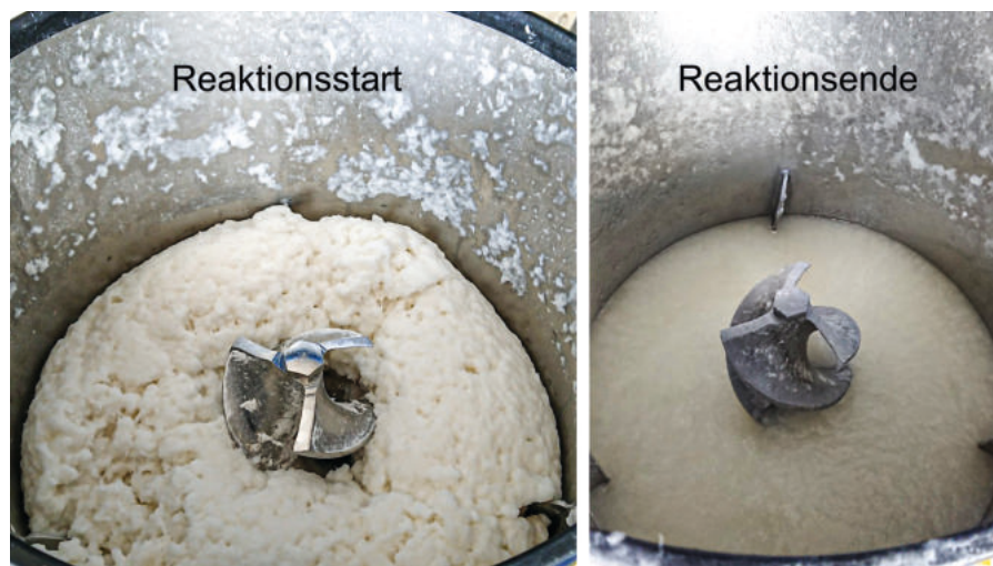
Fig. 3: Pictures showing the preparation of dialdehyde cellulose pulps in the pulper at the beginning and at the end of the reaction, respectively.
