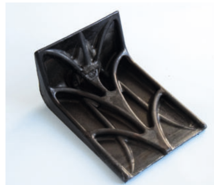
Fig. 4: Demonstrator structure made of rCF hybrid nonwovens (source: Cetex)
