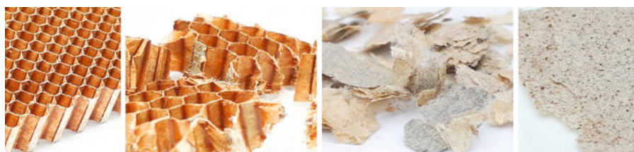
Fig. 1: Used honeycombs become a resource for papermaking – process chain of aramid honeycomb recycling. From left to right: aramid honeycombs, mechanically disintegrated honeycombs or honeycomb cutting waste, phenol resin-free fibre residues after chemical recycling and a fibre mat made thereof.
