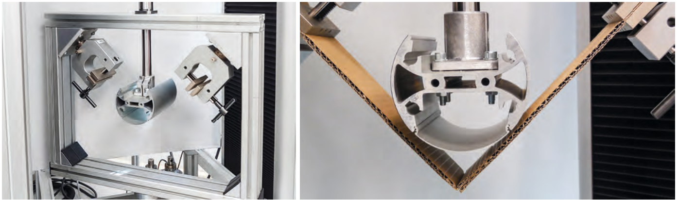
Fig. 1: Test unit for determining the glued seam strength according to FEFCO Test Method No. 55 ©PTS
