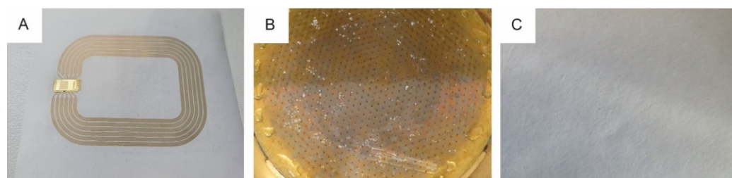
Figure 13. Screen printed RFID antenna with integrated IGZO-TFT microchip (A), 0.7 mm hole reject (B) and sheet adhesion test results (C) of functional screen printed RFID antennas with ‘Loctite ECI 1011’ ink and integrated microchips on Magno Satin substrate.
